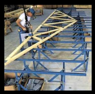
All floor, wall and roof trusses can be fabricated in this workshop, and the house can be framed in a day or two.
